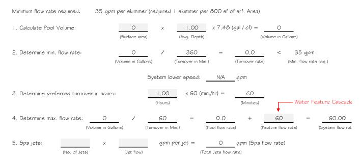
For Single Pump pool/spa combo, use the higher of No. 4 or No. 5 in the following calculations for the pool \$ Spa
